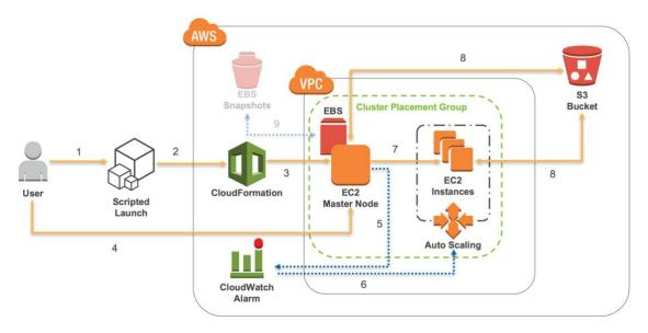
Figure 5: Example template- Based on a tightly-coupled architecture
